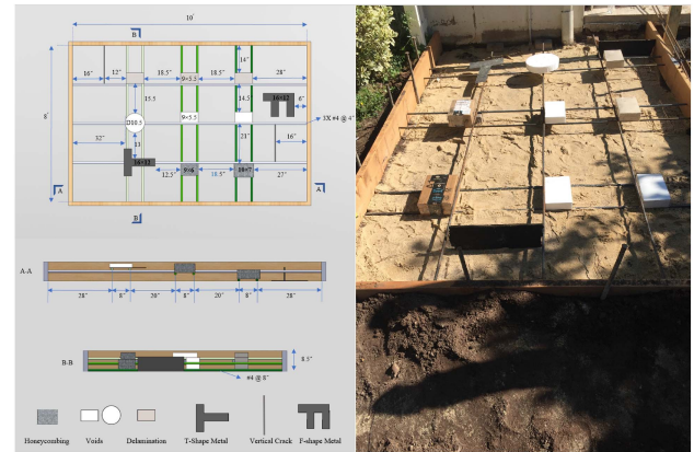
Fig. 7. Ground truth of concrete slab DS2. The left side shows the design of the slab while the right side shows the real slab view before concrete pouring.
